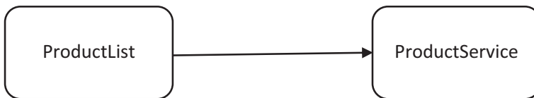
Figure 4-1. Traditional layered approach with tight coupling
